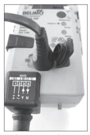
AR, GR, LR, NR, AK, GK, EV, AVK Series Use the interface on the top of the actuator. (Leave all of the wires of the actuator installed.)
